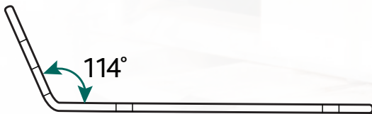
1 SCAFFOLD CLIP, SIDE VIEW SCALE: 1' = 1'-0"
