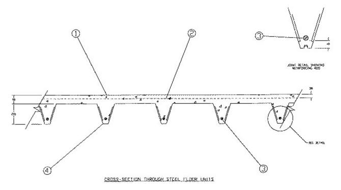
1. **Sand** - **Gravel Concrete** — Normal-density concrete of 2400  $\pm$  50 kg/m<sup>3</sup> density and nominal 30 MPa compressive strength. Minimum concrete topping of D as measured from the top plane of the Steel Floor Units (see Item 4).
