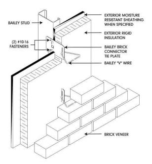
Wind Bearing Steel Stud Wall with Brick Veneer and Shelf Angle (Air Barrier/Vapour barrier Not Shown)
